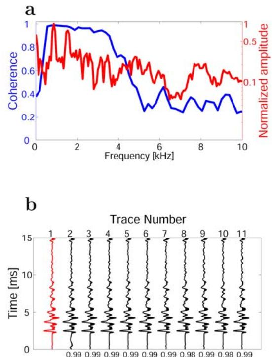
**Figure 3** Results of source repeatability tests. (a) Summed amplitude spectra (red curves, logarithmic scale) and coherence (blue curves, linear scale) for 10 repeat shots. (b) Seismograms from the same 10 shots after 0.5 - 3 kHz filtering. Numbers below the traces are normalised cross-correlation coefficients relative to the stacked master trace shown in red.
