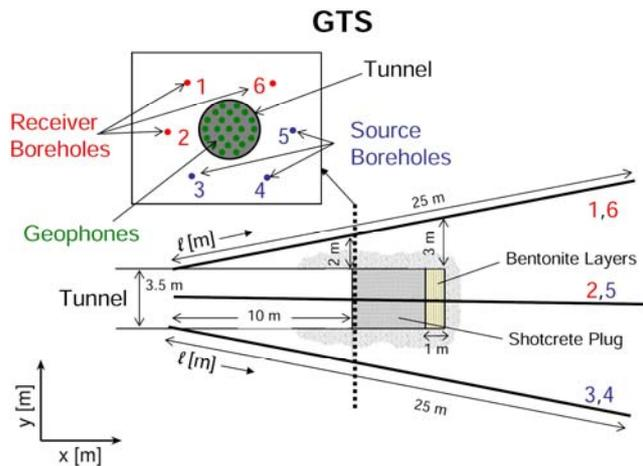
**Figure 1** The Grimsel Test Site experiment setup.
